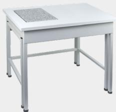
The antivibration table has been designed to eliminate ground vibrations during the operation of automatic feeder. It consists of two separate constructions: the outer, designed to isolate the working part, and the inner. The working part includes a table and a stone separated by a vibration damper. The table features a stone top (located on the left side of the table) and adjustable feet with protective rubber tips, facilitating table levelling on uneven surfaces.
