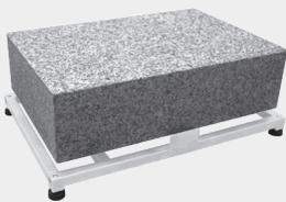
This antivibration table is intended for mass comparators. It is made of powder-coated steel and a massive granite plate placed on top. The table has a safety feature to prevent accidental slipping of the stone, as well as vibration dampening rubbers. Due to low construction, the need to lift large masses to a considerable height is reduced.
