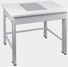
The antivibration table has been designed to eliminate floor vibrations during the operation of PLUS series laboratory balances. It consists of two separate constructions: the outer, designed to isolate the working part, and the inner. The working part includes a table and a stone separated by a vibration damper. The table features a stone top (located at the centre of the table) and adjustable feet with protective rubber tips, facilitating table levelling on uneven surfaces.
