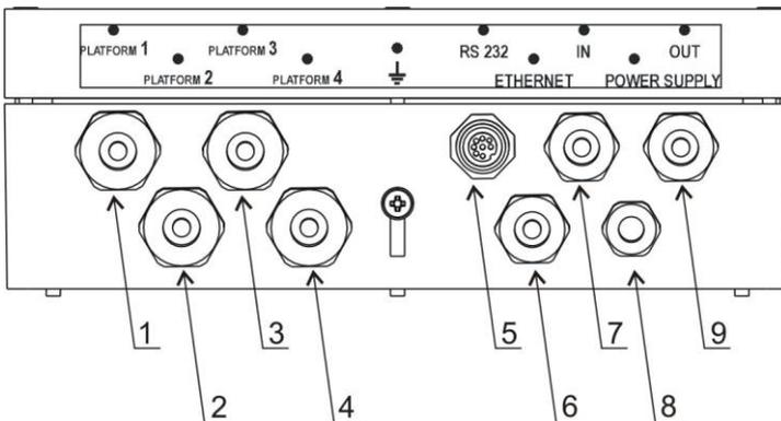
*MW-04 mass converter connectors*
