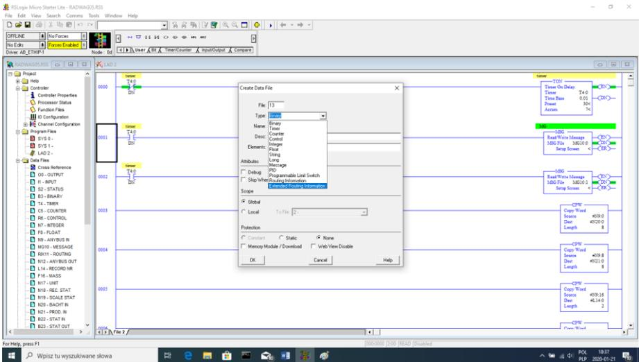
Add also two files of INTEGER type to store data read from the scale and data sent to the scale.
