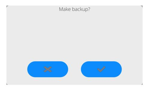
After activating the function, the backup making procedure will be initiated. Throughout the procedure, the balance settings and data saved in the balance memory will be saved in a relevant file.
