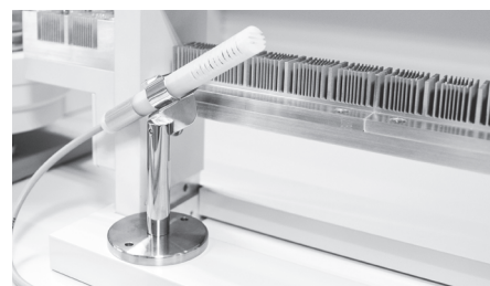
The mass comparator allows real-time monitoring of ambient conditions.
