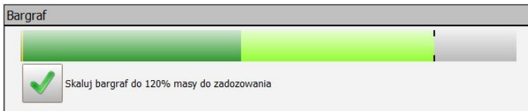
Fig.20 Bargraph for the same amount of mass with a graduation option turned on
