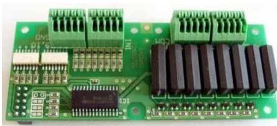
8 inputs / 8 outputs PCB - WE 8
