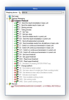
These functions can be presented with reference to particular weighing instruments models.
