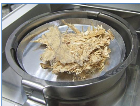
Photo 11. Chipboard – integrated sample (inappropriately prepared material)
