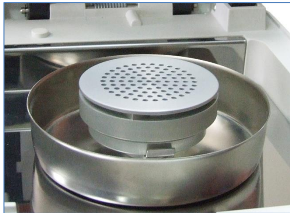
Photo 21. Tester placed inside the moisture analyzer
