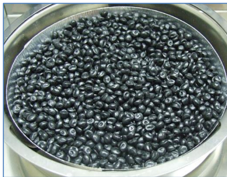
Photo 19. Samples of dark colour = higher drying temperature
