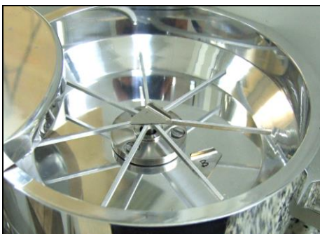
Fig. 23. Balance linearity – testing method 1 linearity point only 500 mg mass standard, (ballast weight is at the bottom of a draft shield)
