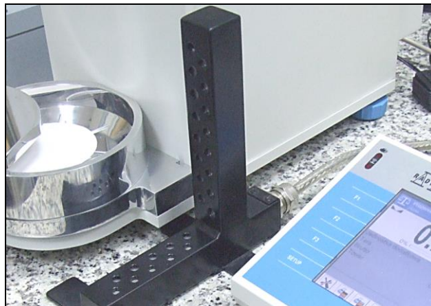
Fig. 30. F series microbalance (for filters weighing) with an ionizer
