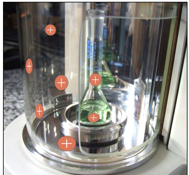
Fig. 16. Unbalanced electrostatic charges
