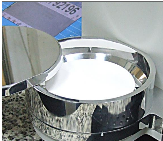
Fig. 14. MYA 5.3Y/F – cellulose filter of 90 mm diameter
