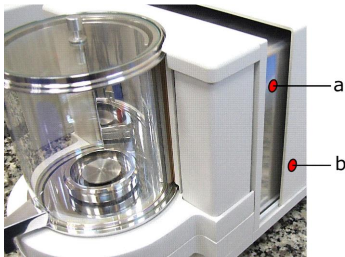
Fig. 5. Microbalance design, weighing module external (b) and internal housing (a)
