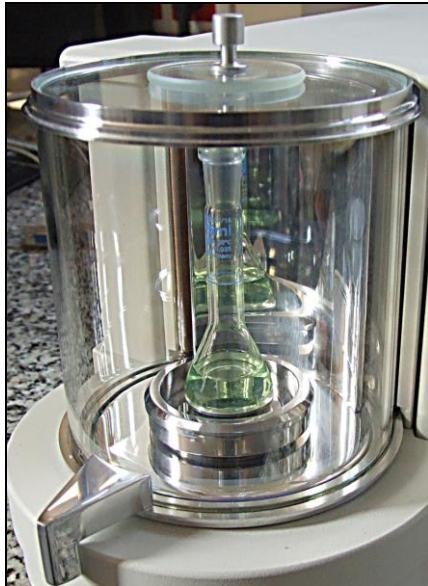
Fig. 31. Weighing liquid by means of vessel with a tapered inlet, liquid evaporation in course of weighing limited
