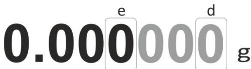
Figure 14. Microbalance MYA series - verification unit (e) and reading unit (d)
