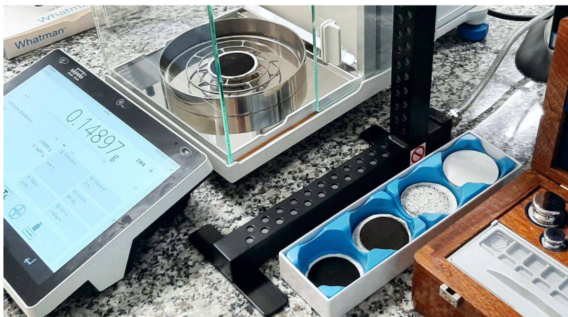
Figure 18. Static electricity in filter mass measurement – Ionizer DJ-04
