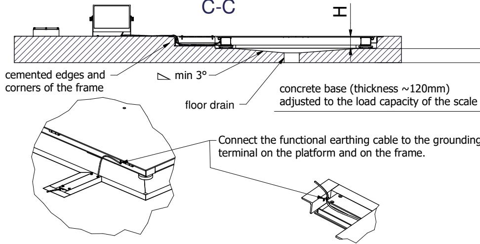
Equipotential circuit - connect indicator, power supply and frame with the platform.
