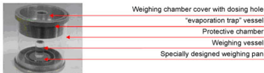
Fig. 10 Kit for checking pipettes on RADAG balances series AS and XA/X
