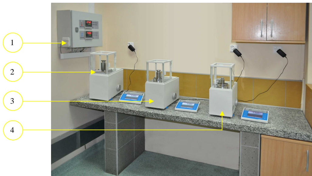
Fig. 5 Measuring workstation for manual testing of a mass comparator
