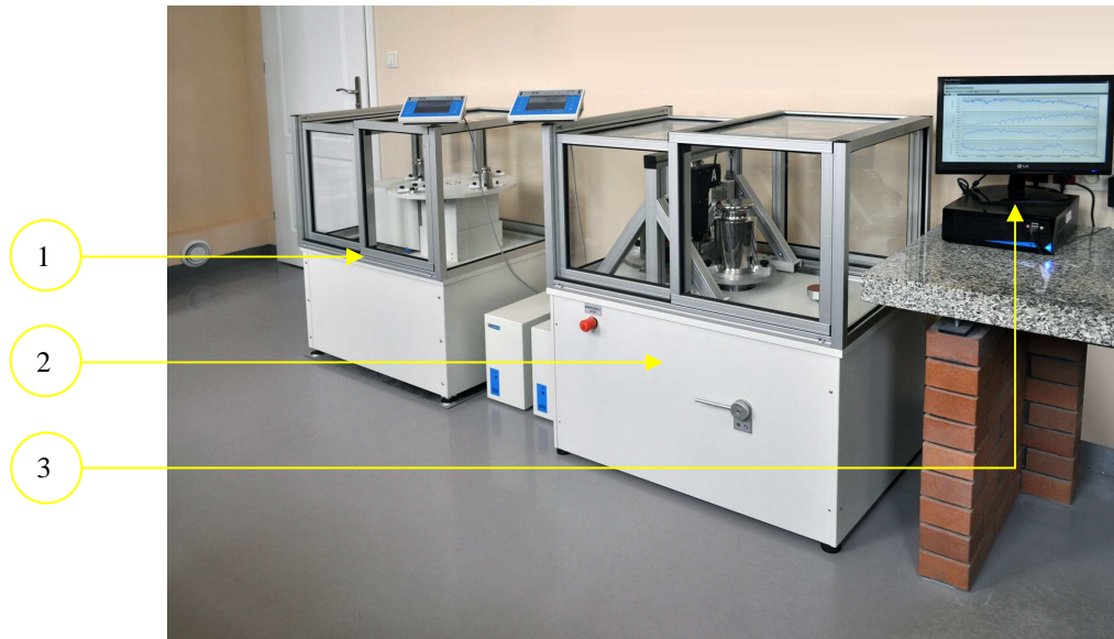
Fig.9 Measuring workstation for automatic testing of mass comparators
