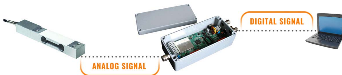
Fig. 29 Connection diagram of MW-01 strain gauge weighing cell module
