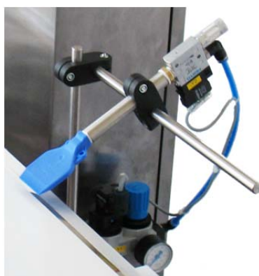
Fig. 91 Rejection system using compressed air
