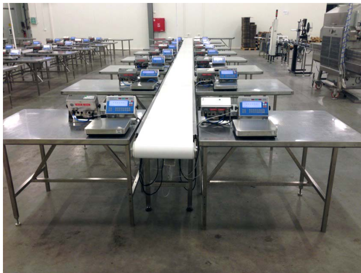
Fig. 50 Production hall, workstations for dosing fish to cans
