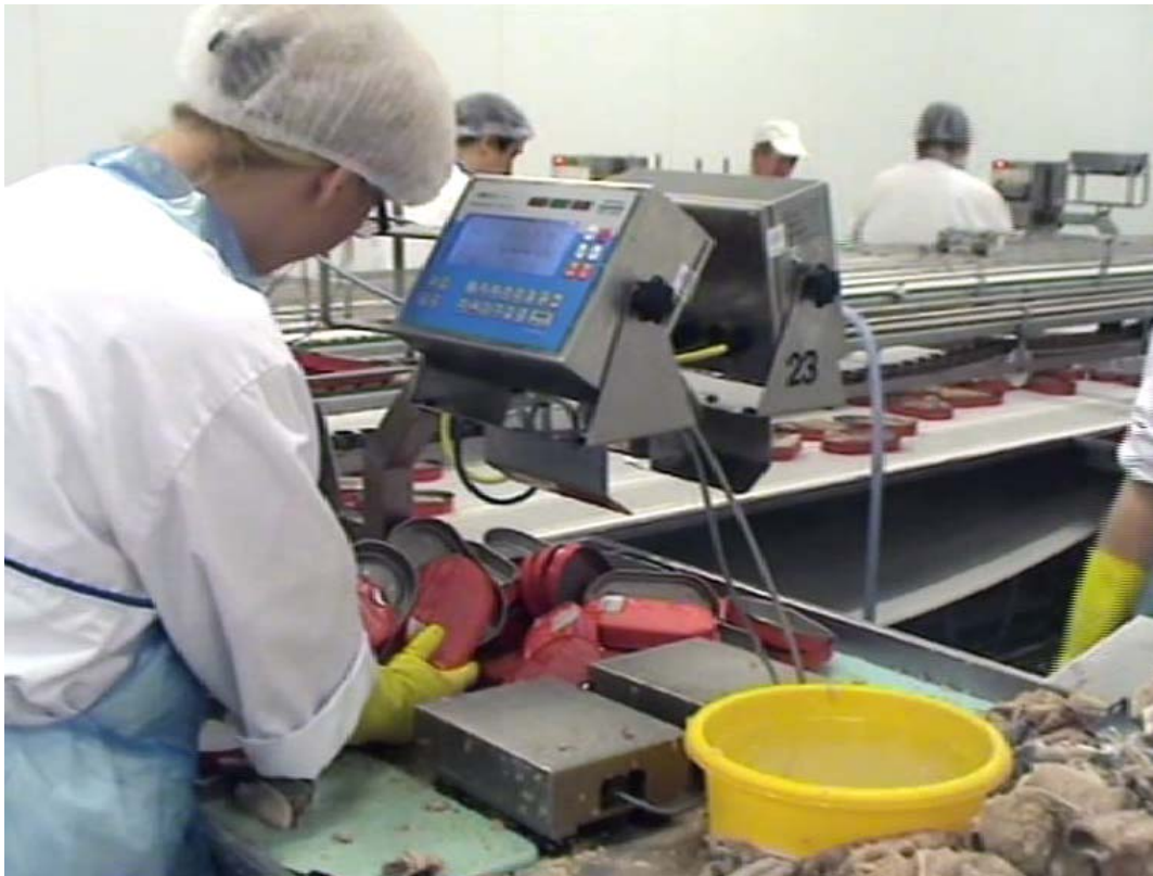
Fig. 53 Weighing workstation on fish dosing line
