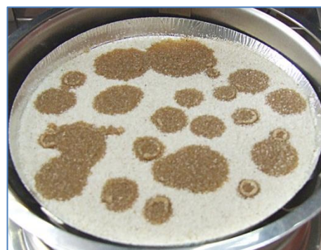
Photo 16. Sebonamine sample dried with use of silica sand (ca. 2.2 % of dry mass)
