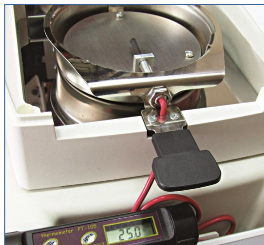
Photo 3. Control thermometer used with MA.R/MA.3Y moisture analyzers (available from November 2012)
