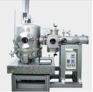
For a vacuum comparator, the temperature range must be constant throughout the entire operation time of the comparator. Temperature changes greater than the  $\pm 0.1$  C range cause significant increase in the zero drift as well as the repeatability of the comparator, as can be seen from the graph even 5-6 times.
