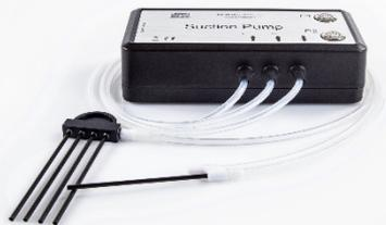
The pump draws water from four measuring vessels at the same time. The procedure time is reduced from 6 hours to 1 hour.
