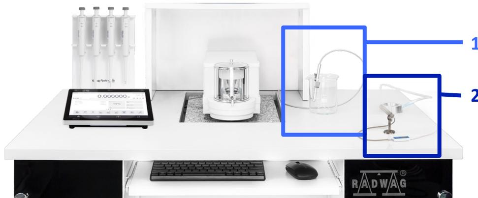
1. Water temperature measurement probe
