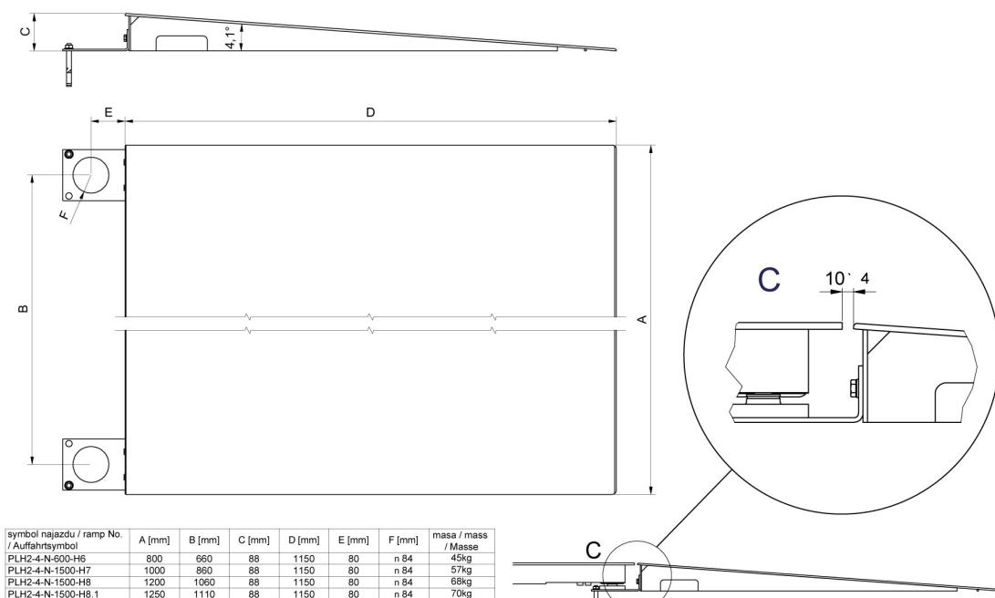
Ramps made of stainless steel
