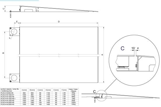
Ramps made of stainless steel
