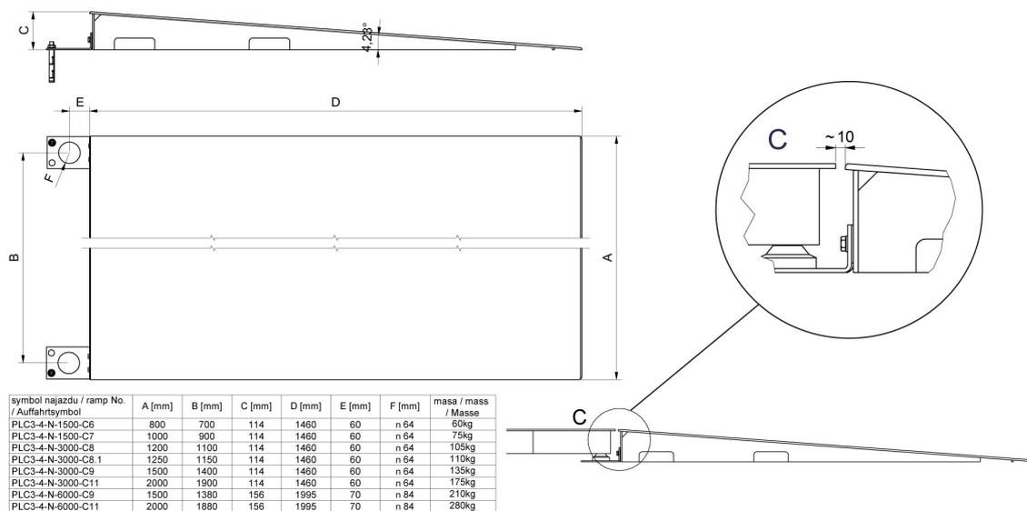
Ramps made of powder-coated steel
