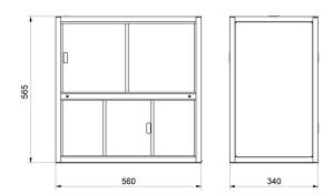
Anti-draft chamber for WAY-KOmass comparators
