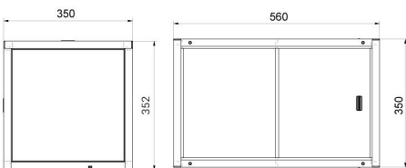
Anti-draft chamber for XA 5Y / XA 5Y.A balances
