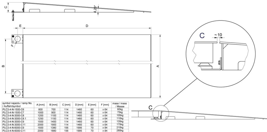
Ramps made of powder-coated steel
