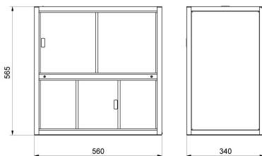
Anti-draft chamber for WAY-KO mass comparators
