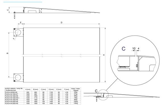
Ramps made of stainless steel
