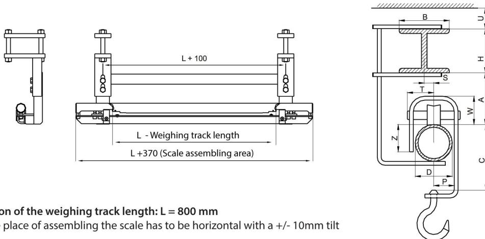
Dimensions of an overhead track scale with a shaft of  $\varnothing 60$  (standard version)
