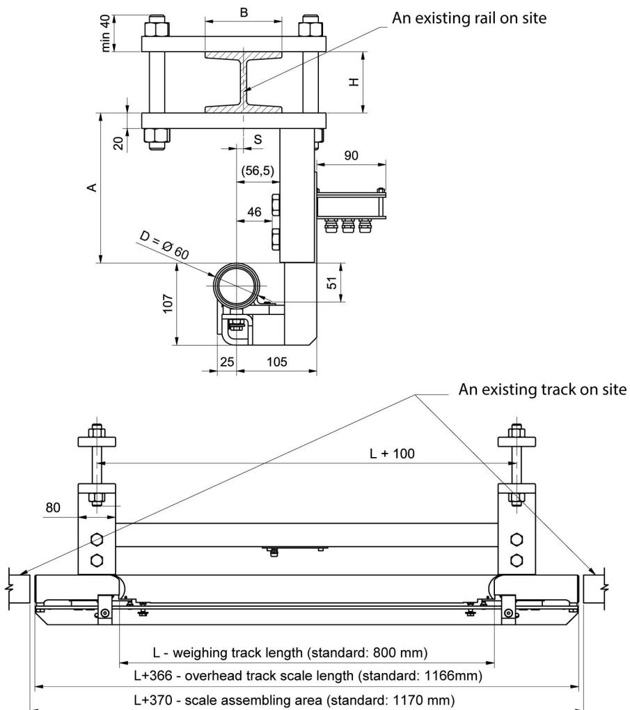
Minimum track clearance:  $A = 90 \text{ mm}$ .
